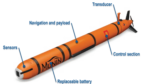
Figure 12 – The Munin – an Autonomous Underwater Vehicle (AUV), which is about 3.5m in length and was used for very high resolution seabed mapping
