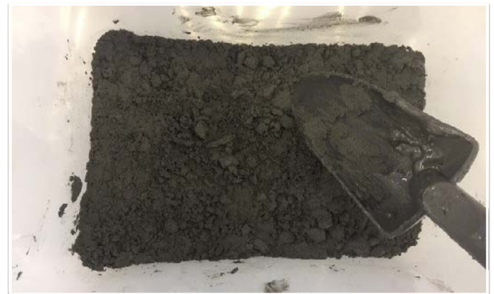
Figure 3 – An example of fine sand tailings
