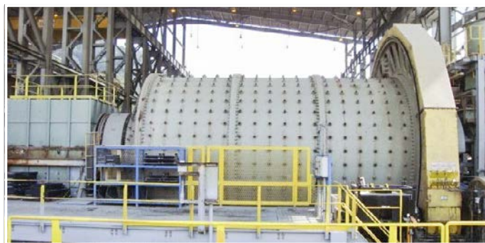
Figure 1 – Ball mill used to grind ore
