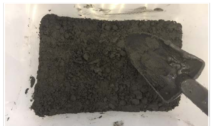
Figure 3 – An example of fine sand tailings
