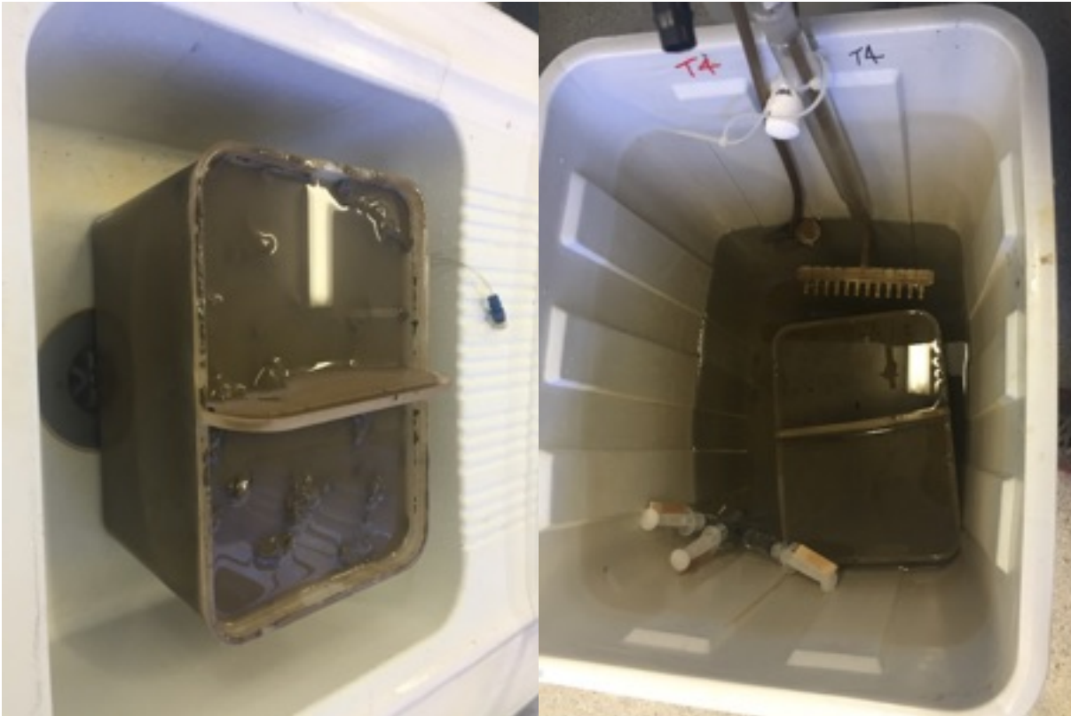
Photos 1-2: Treatment T1 ready for bivalve removal for bioaccumulation assessment. T4 with water drawn down, Rhizon sampling, prior to bivalve removal for bioaccumulation assessment.
