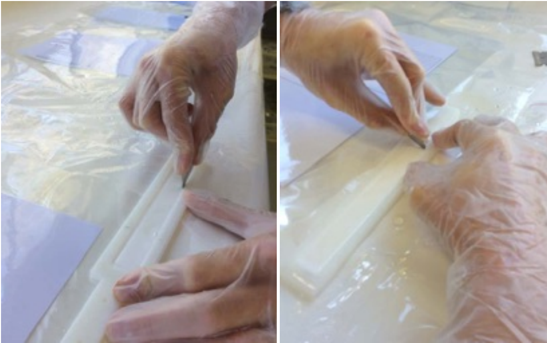
Photos: Using a scalpel to cut through the filter membrane and gel layers from the open window.
