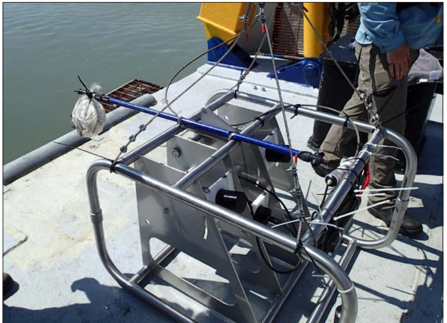
Plate 2.5 Bait bag affixed to UIS during BRUV deployments
