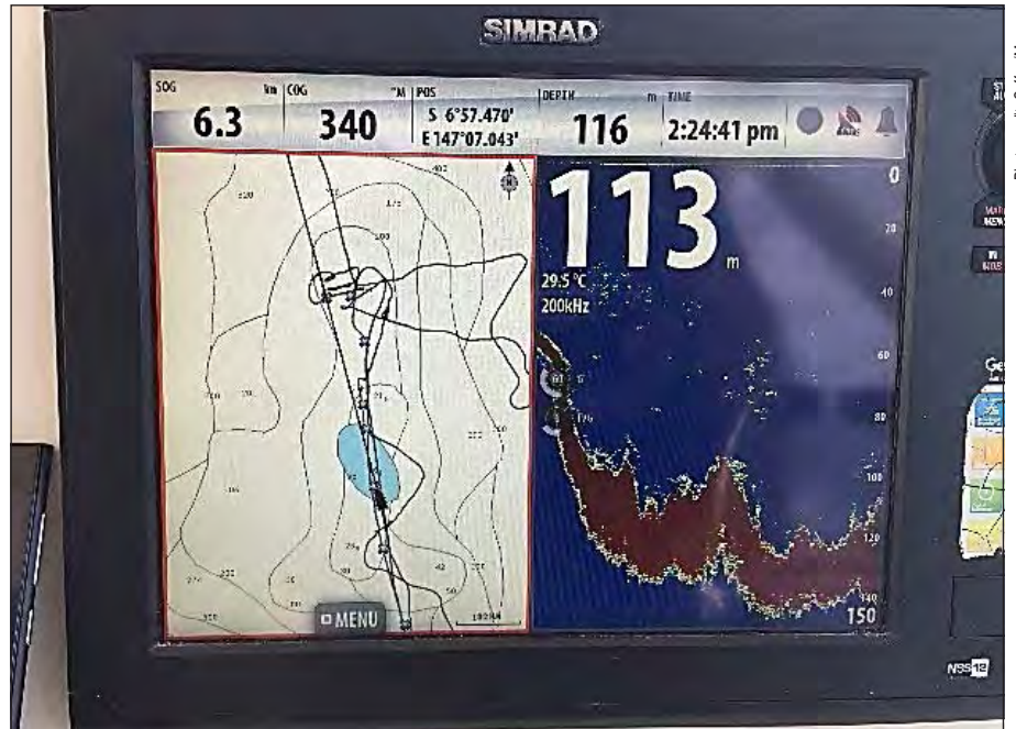
Plate 2.5 GPS-coupled Simrad NSS12 plotter
