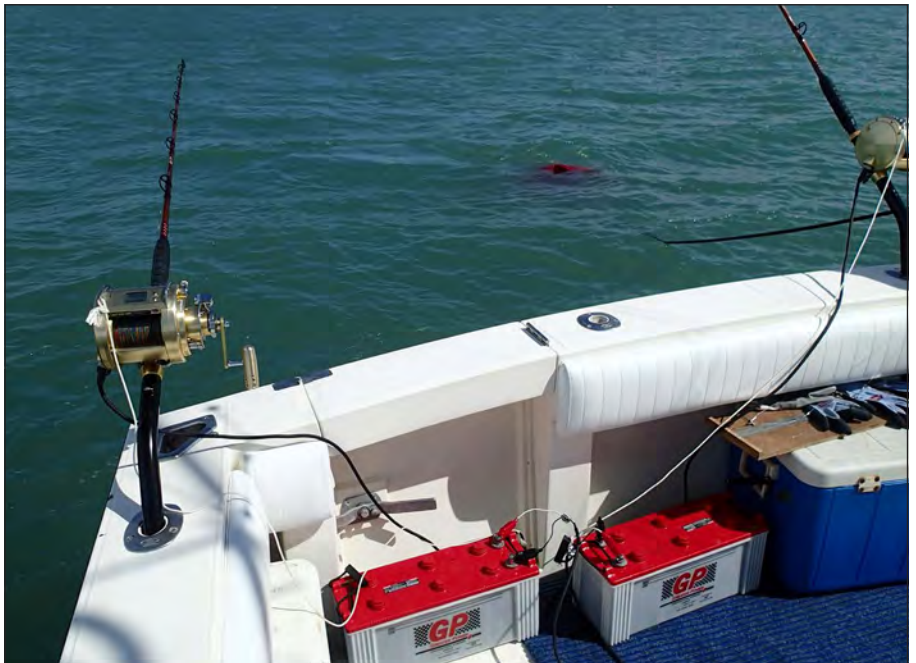
Plate 2.2 Electric reels connected to 12V deep-cycle batteries
