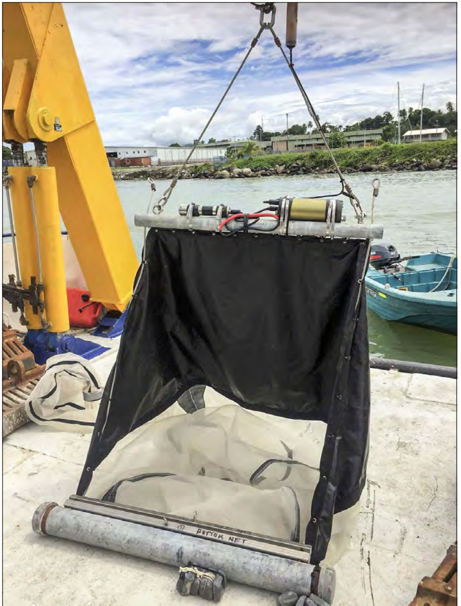
Plate 2.8 Tucker trawl system equipped with single 1,000 micron mesh net used to collect micronekton during the 1 May 2017 survey. Hardware attached to top frame corresponds to Valeport pressure sensor to monitor trawl depth.
