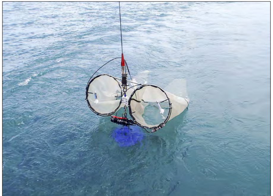
Plate 2.2 500-micron ( \mu\text{m} ) mesh Bongo sampler (nets A and B) used for zooplankton sampling
